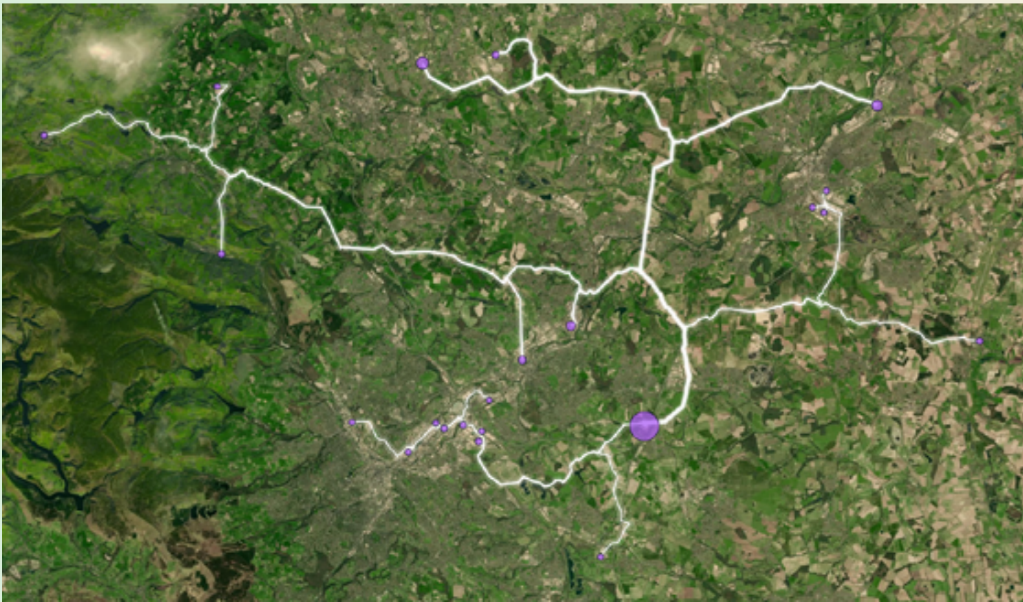
Figure 2: Least cost hydrogen network for 21 emitters in the South Yorkshire region, found using routing software AENi. The largest dot represents a hydrogen electrolyser plant sited at the Thurcroft Grid Supply Point (400 kV transmission). Credit Joseph Hammond of AENi.
